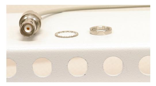
2. Insert the cable end of a BNC connector assembly through a BNC mounting hole so that the BNC connector mounts from the front of the cover (8121-2461, parts list item 7).
