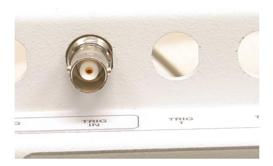
3. Slip the lock-washer and nut over the threaded portion of the BNC connector protruding through the front of the cover (2190-0102 item 8 and 0590-1251
