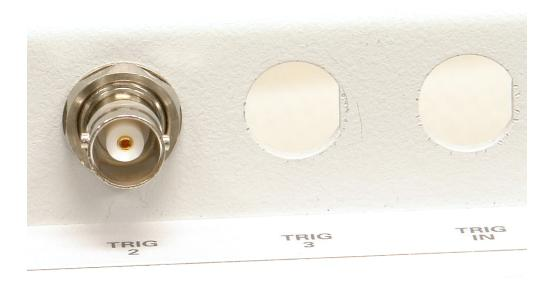
4. Tighten the nut to the lock-washer on the BNC connector using a 9/16 wrench to 35 inch-pounds.
