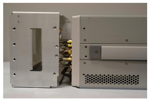
2. Slide the Y1270A frame onto the M9018A chassis using great care not to pinch the cables running between the Y1270A frame, and the M9018A chassis.
